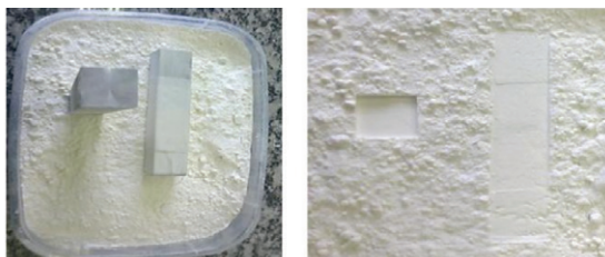
Figure 1: Deformations caused by the parallelepiped supported on the major and minor faces
