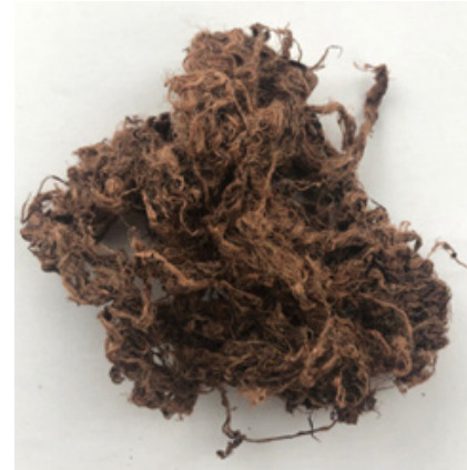
Figure 6 - Fibers after second boiling, before washing again to remove remaining impurities
