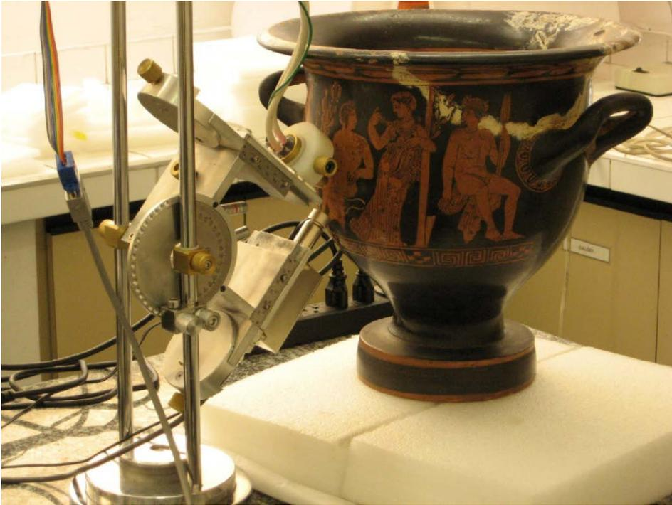
Figure 3: Portable X-ray fluorescence system positioned for a measurement.
